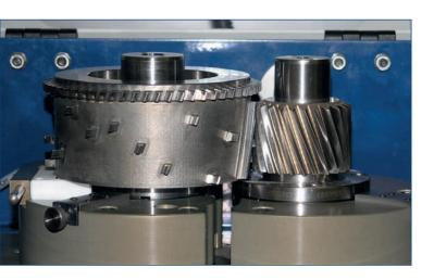
Depending on the number of teeth and the device, the entire gear profile can be scanned within 3 to 13 minutes. It is possible to evaluate a large number of other parameters, besides the usual parameters, such as profile, pitch and runout, with the measuring time remaining the same.
